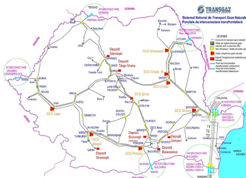
Figure 1 - Map of the National Gas Transmission System and the NTS cross-border interconnection points
